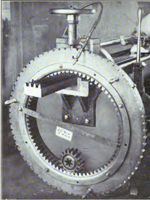
FIG. 50.—Broaching a 22-in. internal gear.
